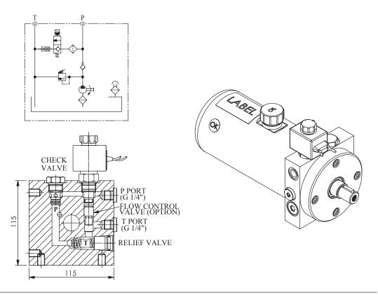
The W81BT mini power pack series is designed for use with belts powered by various engines. These mini power packs have been designed mostly for agricultural use, but can be used in other fields.
