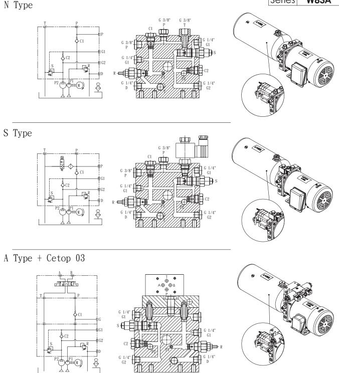
The W83A series power pack is designed for applications that need high pressure and larger flow, but use a low-power A.C. motor. The power pack uses a special manifold (W800553). All screw-in cartridge valves have been designed to be adjusted easily to service the power pack quickly. They still have the same dimensions and functions as the standard manifold (W800532). Our standard AC motors range from 0.25HP to 3.0HP.
