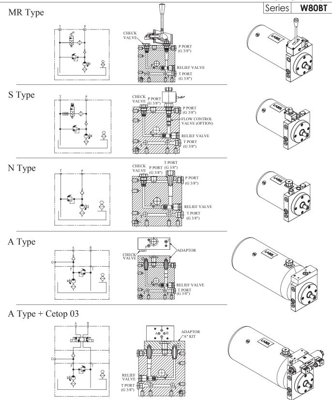
The W80BT power pack series is designed for use with belts powered by various engines. These power packs have been designed mostly for agricultural use, but can be used in other fields.
