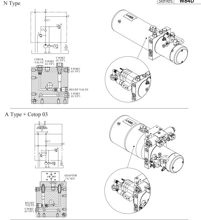
The W84D series power pack is designed for applications that need high pressure and larger flow, but use a low-power D.C. motor. Because the power pack uses a standard manifold(W800532), they will have the same functions as the W80D series power pack.
